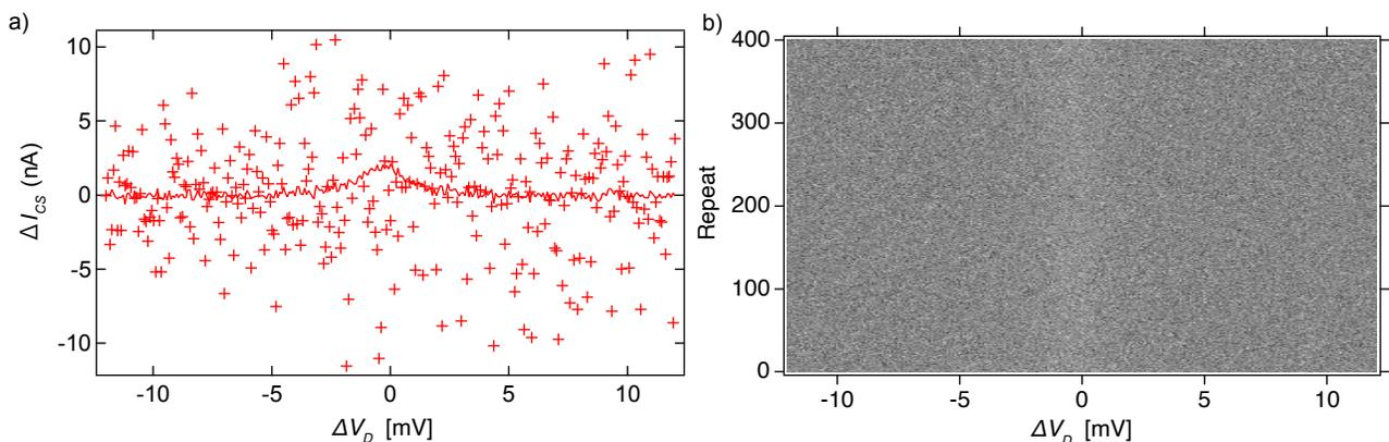
FIG. S4. a) Markers illustrate a single measurement across the charge transition, which takes 30 seconds to complete. No peak in  $\Delta I_{CS}$  can be seen in this raw data. After averaging 400 of such scans together (solid line), however, a small peak in  $\Delta I_{CS}$  is seen at  $\Delta V_D = 0$ . b) Raw  $\Delta I_{CS}$  data (greyscale) for 400 scans as in panel a). Averaged together, they yield the solid line in panel a).
