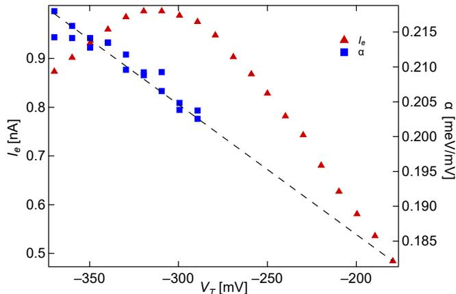
FIG. S3. Variation of lever arm  $\alpha$ , and charge step  $I_e$  measured independently over the full range of  $V_T$  explored in this experiment. Dashed line: extrapolation of  $\alpha$  into the strongly-coupled regime where it cannot be measured directly.
