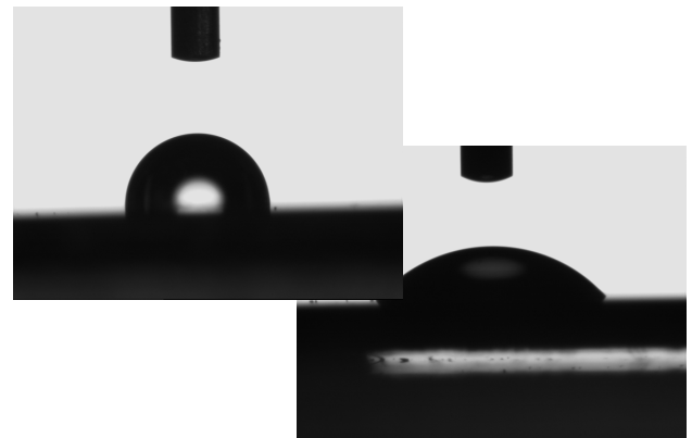
Figure 2: Effect of plasma treatment on water contact angle
