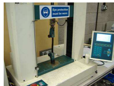
Figure 3: Adhesion test (Lap Shear Strength) machine and schematic
