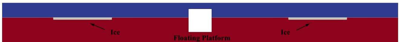
Figure 1: Layout of the structure-ice-wave tank
