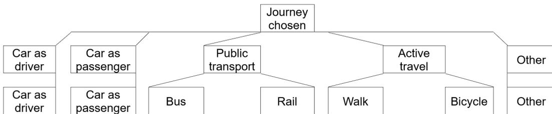
Figure B.16: Tree structure specified for nested logit regression model
