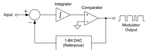
Block diagram of 1-bit delta-sigma modulator
