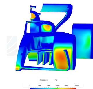
Figure 6: Air pressure distribution along car with halo
