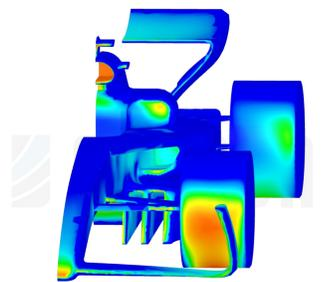
Figure 8: Air pressure distribution along car with no halo
