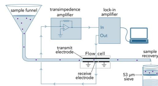
Fig. 4. Impedance Spectrometer Design [2]
