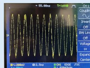
Fig. 5. Frequency produced by PC. 400 Hz input.
