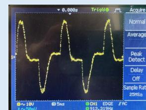
Fig. 6. Frequency produced by MacBook. 400 Hz input.
