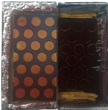
*Figure 1. One of the cells used for testing, Left: Back contact, Right: Front*
