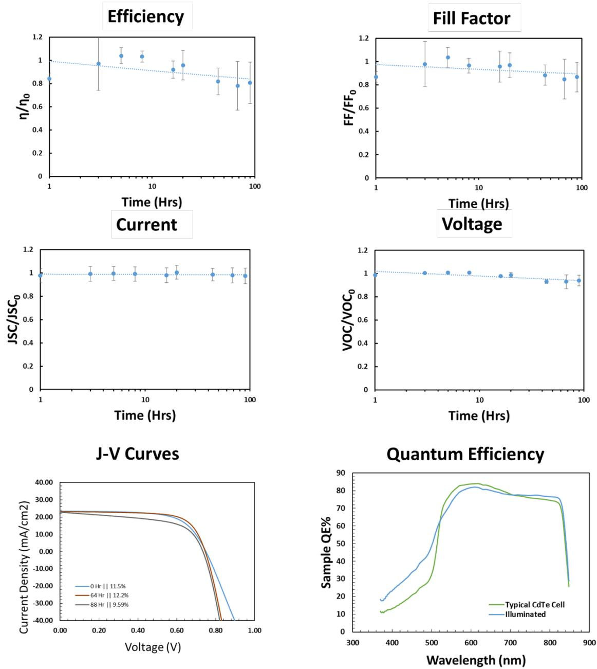
Figure 4. Summary of Cell Characteristics under Illuminated Conditions
