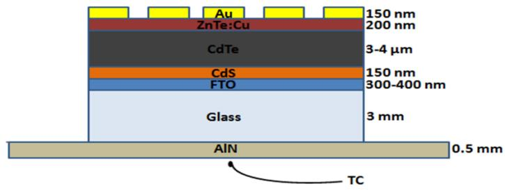
*Figure 2. Cross section of Solar Cell*
