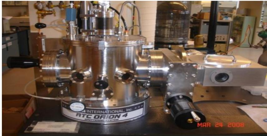
Figure 3: Sputter deposition chamber
