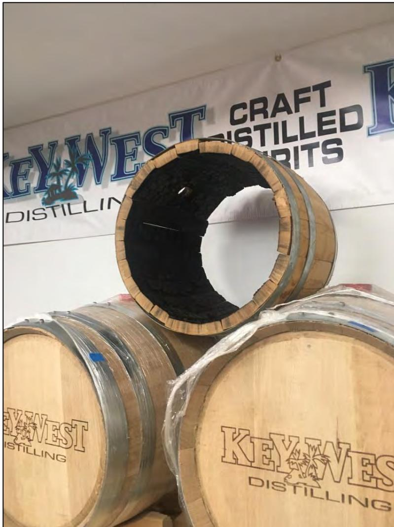
**Figure 19:** Inside view of charcoal flamed barrels for storing either rum or whiskey
