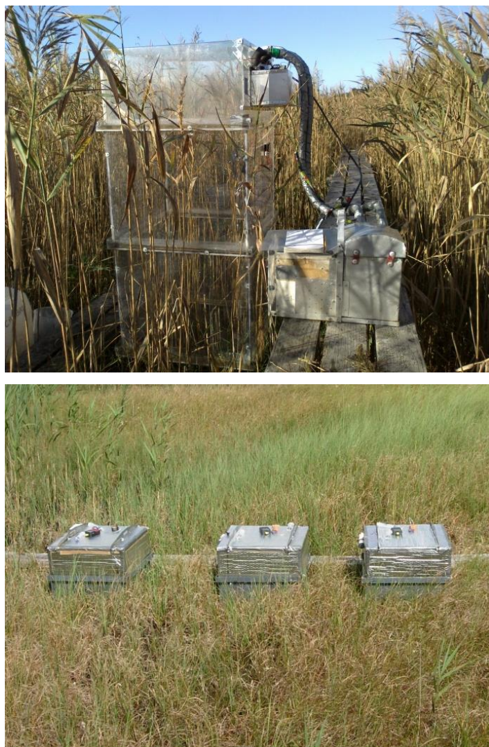
Figure 4.16. Static chambers used for the measurement of carbon dioxide (upper) and methane/nitrous oxide (lower).
